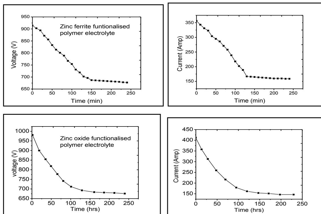
**Fig. 6 Discharge characteristics of electrochemical cell.**
