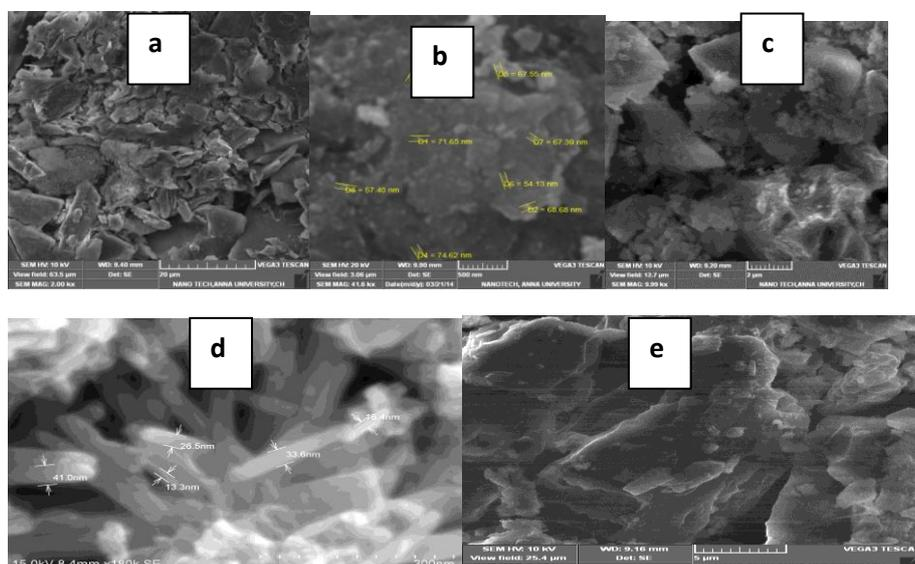
**Fig 4. SEM images of a) supramolecular polymer, b) zinc ferrite nanoparticles c) zinc ferrite/solid polymer electrolyte d) nano zinc-oxide and e) zinc oxide/solid polymer electrolyte**
