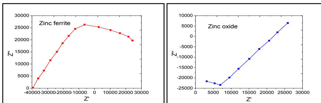
**Fig. 5 Nyquist plot region of zinc ferrite/oxide doped supramolecular polymer composites**
