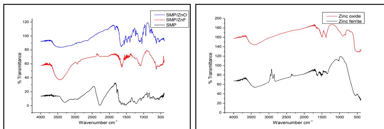
**Fig 1. FTIR spectra of supramolecular polymer, ferrite/oxide nanoparticles and supramolecular polymer composites**
