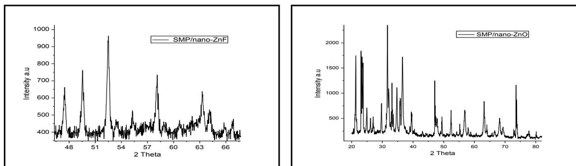
**Fig 2. XRD patterns of zinc ferrite/oxide doped supramolecular polymer composites**
