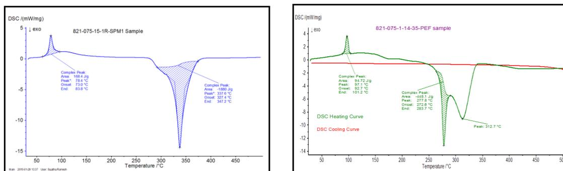
**Fig 3. DSC thermogram of zinc ferrite/oxide functionalized supramolecular polymer electrolyte**
